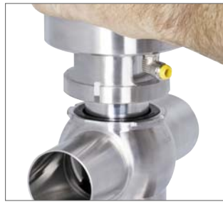
Turn actuator clockwise through 90° and pull valve insert out
