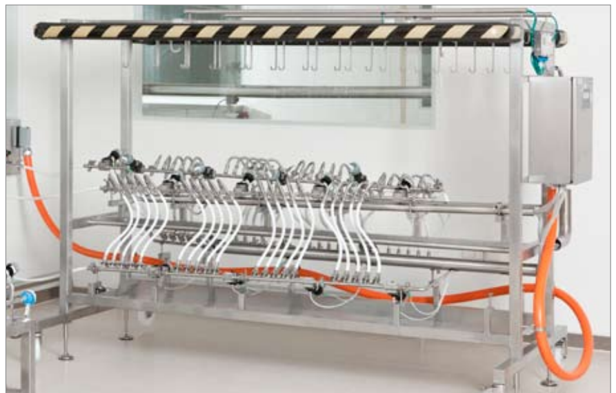
The process trolley and the media panel form the centerpiece of the new product formulation line, where weighing and metering of all formulation components take place.
