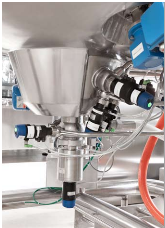
Instead of the classic, central tank-bottom valve, three tank-bottom valves of the VESTA® series were installed, two of them laterally at the cup-shaped tank wall, another centrally at the bottom.
